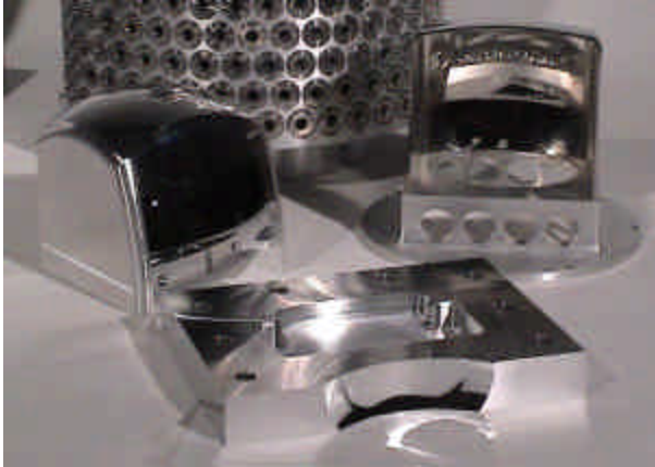
Figure 4: Electroformed Telescope Hardware
